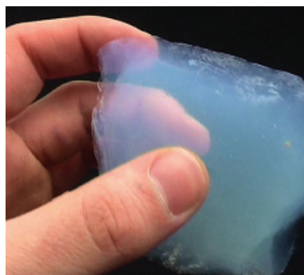
Silica aerogel produced by Steve M. Jones, NASA Jet Propulsion Laboratory. (Courtesy of Zoe Laughlin.)
