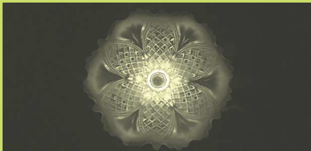
Fluorescence picture of a uranium glass fruit bowl. (Courtesy of Jake Baum and a residency at Monash University, School of Physics and Materials Engineering.)
