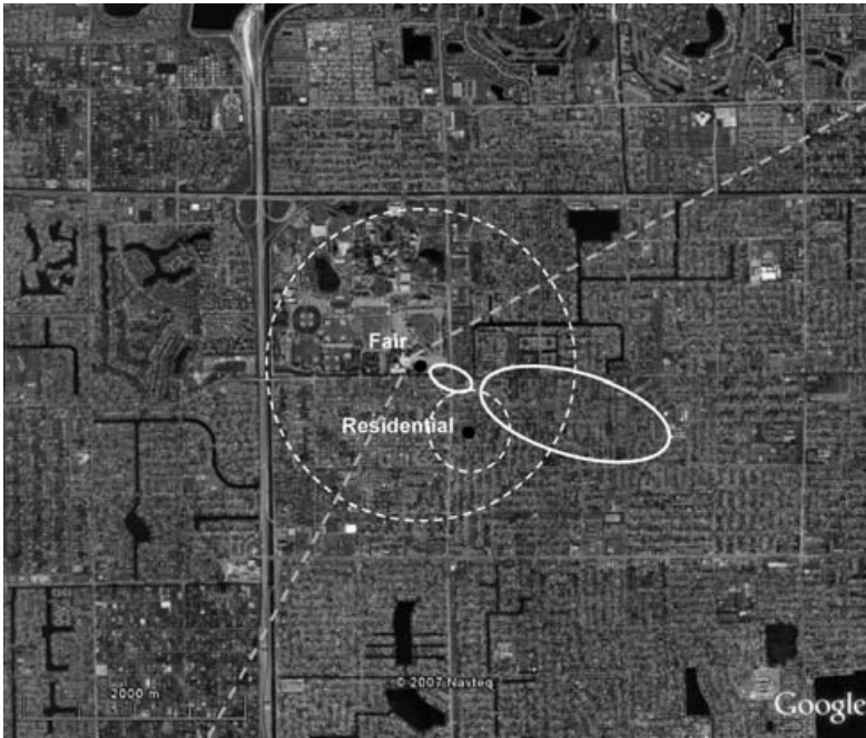
Fig. 1. Aerial photograph of the Miami suburban site including the location of the Fair and Residential towers, their radiation (circular) and turbulent (elliptical) source areas and the accepted sector for flow (60 to 210 degrees, dash-dot lines). The larger turbulent footprint is a stable (end of night) case and the smaller one is an unstable (afternoon) case.
