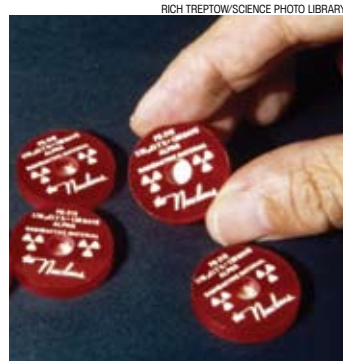
Polonium-210 discs. This isotope of polonium is a powerful emitter of alpha particle radiation.
