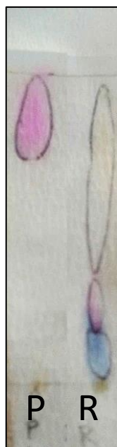
Figure 1. TLC sheet containing pink (“P”) and red (“R”) dye.
