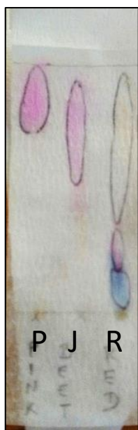
Figure 4. TLC sheet containing pink dye (“P”), beetroot juice (“J”) and red dye (“R”).
