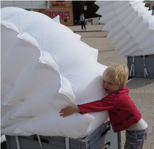
Because they are made from fabric and not hard material they are called 'soft robots'.
