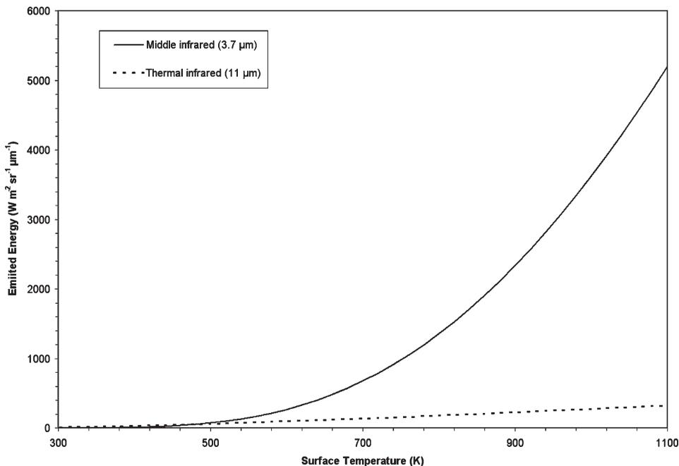
Figure 2. Thermal output from surfaces at MIR and TIR wavelengths modeled according to Planck's Radiation Law.
