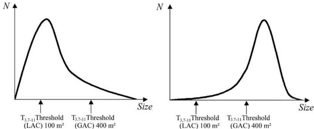
**Figure 8.** Theoretical fire size distributions for two different ecosystems. As illustrated here, assuming a constant fire temperature, application of any particular  $T_{3.7-11}$  threshold to AVHRR data of these areas will directly translate to a minimum detectable fire size for that ecosystem, with this size being 4 times larger for GAC data than for LAC data.
