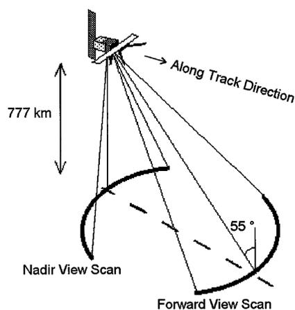
**Fig. 2** The viewing geometry of the ATSR sensor, mounted onboard the orbiting ERS spacecraft. Every 150 ms the sensor makes two scans of the Earth's surface. The nadir-view scan views at zenith angles 0–22°, the forward-view scan views at zenith angles 53–55°. As the satellite moves along the orbit track each ground location is imaged in both the nadir and forward views
