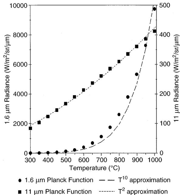
**Fig. 4** The relationship between emitted radiance and brightness temperature for the ATSR 1.6- and 11- $\mu\text{m}$  channels, calculated using the Planck function (Eq. (1)). The dashed lines show the relationships obtained if the Planck function is approximated by Eq. (2)
